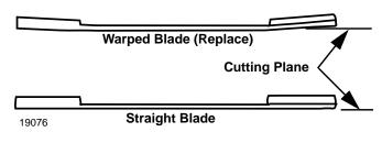
Comparison of Warped and Straight Blades Figure 4-14
